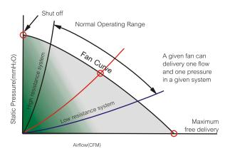
This non-linear expression of airflow versus static pressure can be stated as:
